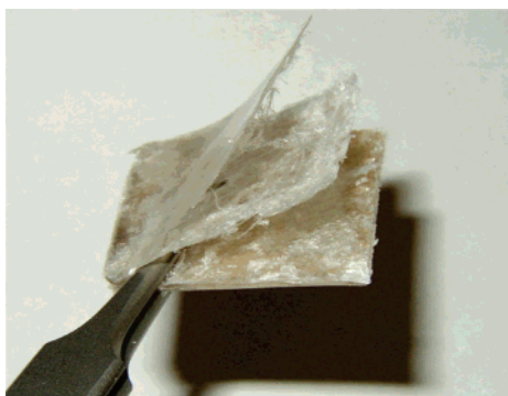
Figure 12. A sheet of polystyrene peeled from the outer surface of an injection molded PS/2% GC11BS plaque.
